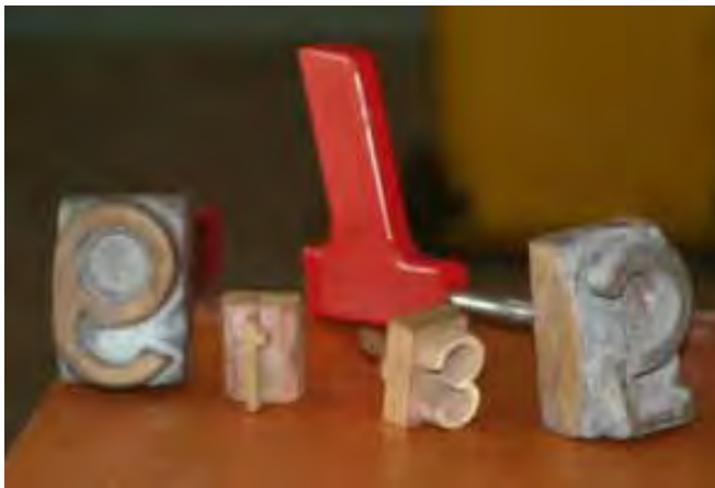
Figure 2. Two different types of freeze branding iron. The large numbers are 3" tall, have a particularly heavy backing block. Because of their size, they are more suited to cattle or adult horses, but only need to be applied for 5-10 seconds. The smaller numbers are 1 1/2" tall, and fit into a handle with a backing plate that holds several numbers. This allows multiple numbers to be applied in a single brand application. These particular irons are applied for 12 seconds for a coloured horse, and at least 20 for a grey.
